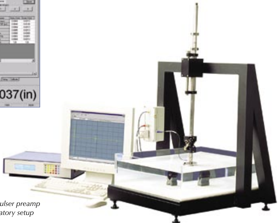
Thickness of a multilayer plastic bottle measured with a 5900PR using a V2064, 125 MHz delay line contact transducer and ScanView Plus TC software
