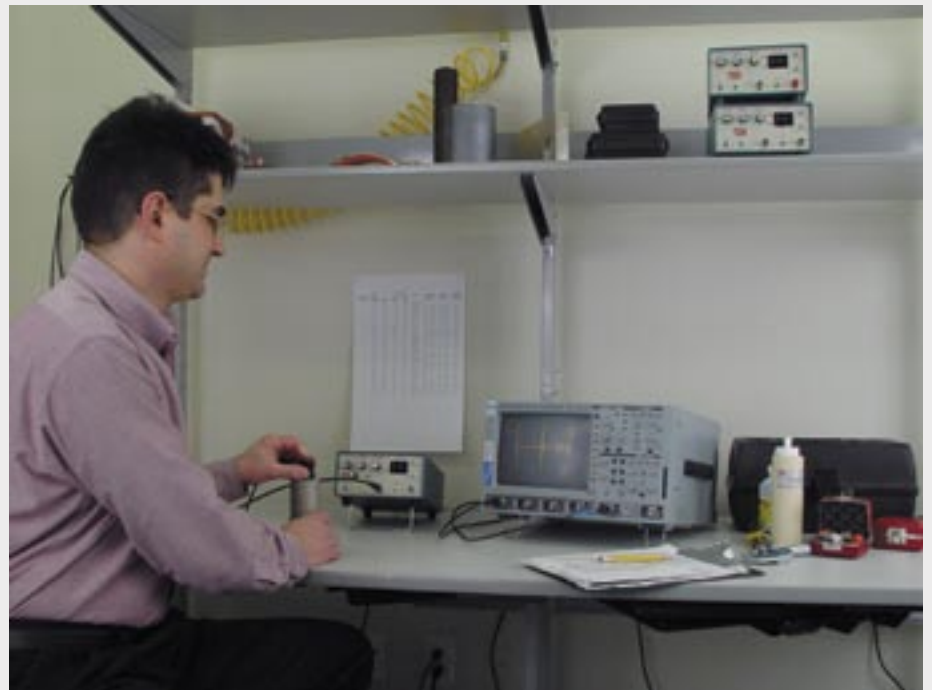
Model 5077PR square wave pulser-receiver used in conjunction with a digital oscilloscope for pulse-echo ultrasonic measurements of material characteristics.
